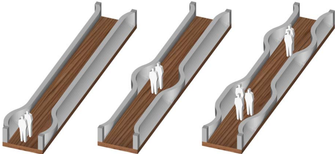
Figure 17. A corridor can adapt to passing people. The width of the corridor with a plan width of two meters expands from 1.40 meter to 2.60 meters.
